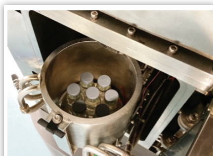
Figure 1. Inner cylindrical chamber of the LyoCapsule™ Freeze Dryer with temperature-controlled shelf and wall.
