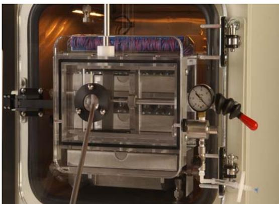
**Sample Thief - for removal of vials during secondary drying**
