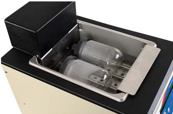
**Flask Shell Freezing in a Shell Bath**
