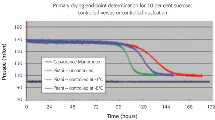
Figure 1: The end of primary drying where the Pirani gauge converges with the Capacitance Manometer (5)
