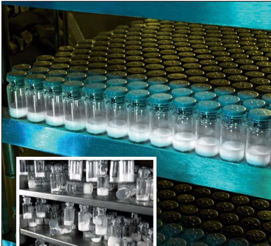
*West FluroTec® on the top of elastomeric stoppers can eliminate sticking of stoppers to shelves in lyophilization chambers.*
