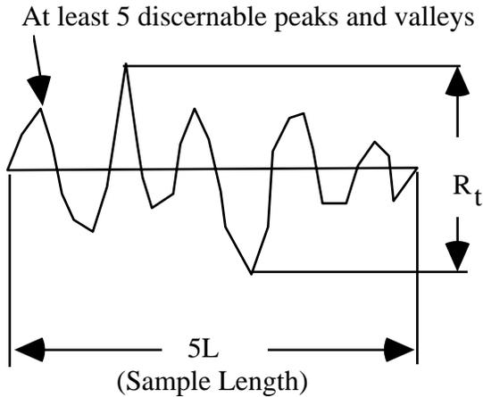
As seen in the diagram,  $R_t$  tends to give less variance in readings because it takes the highest peak and lowest valley out of five peaks and valleys. On the other hand, no less than five different  $R_y$  readings could be obtained from the above surface.
