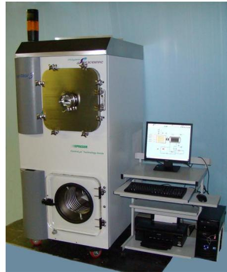
**Figure 4.** LyoStar 3 with ControlLyo™ Nucleation On-Demand Technology
