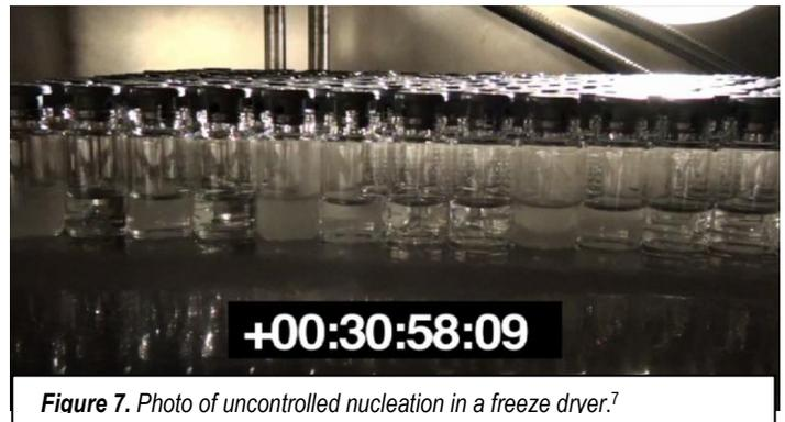
**Figure 7.** Photo of uncontrolled nucleation in a freeze dryer.<sup>7</sup>
