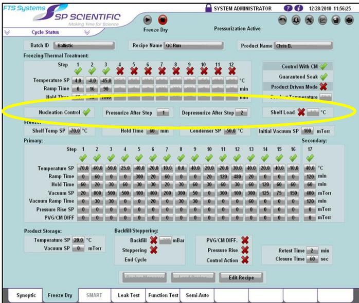
**Figure 5.** LyoStar 3 Lyos Software with *ControlLy*<sup>TM</sup> Nucleation On-Demand Technology
