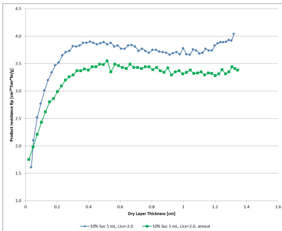
Figure 4: Impact of annealing on product resistance
