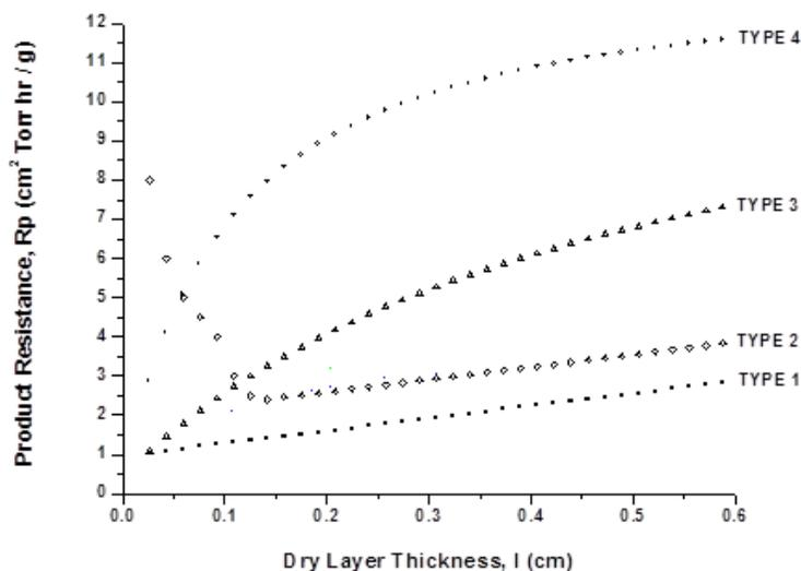
Figure 1:  $R_p$  behavior as proposed by Pikal<sup>3</sup>
