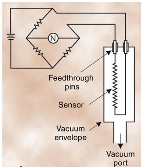
A Pirani gauge works on the principle that when a heated metal filament is suspended in a gas, it will lose heat to the gas molecules as they collide with the wire. If the gas pressure is reduced, the number of molecules present will fall proportionately and the wire will rise in temperature due to the reduced cooling effect.
