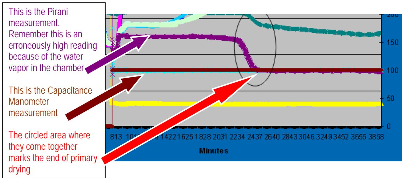
The advantage of this method is that it is non intrusive and it can be utilized on any freeze dryer that is equipped with both a Pirani gauge and a capacitance manometer pressure gauge. The disadvantage is that it becomes harder to see a differential when very low water vapor flows are present. Another disadvantage is that the Pirani adds a heated element to the inside of the freeze dryer which may be an issue if the product being freeze dried has a high flammable solvent content.
