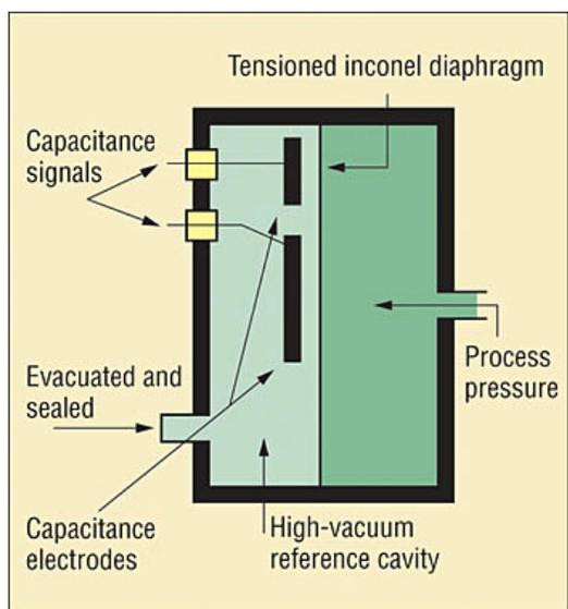
As system (process) pressure changes, there will be a change in pressure on the diaphragm causing the diaphragm to move. There will be a direct correspondence between pressure input and voltage output as the distance between the diaphragm and the electrodes changes. A typical capacitance manometer's signal conditioning electronics will provide an output varying from 0 to 10 volts with a linear relationship between output voltage and pressure.
