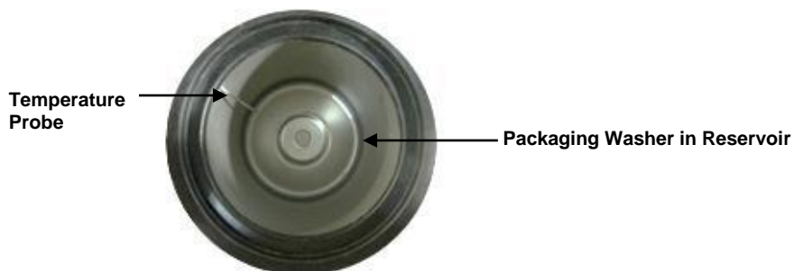
HC80-1 Reservoir (Top View)
