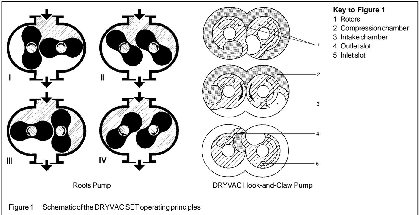
Figure 1 Schematic of the DRYVAC SET operating principles
