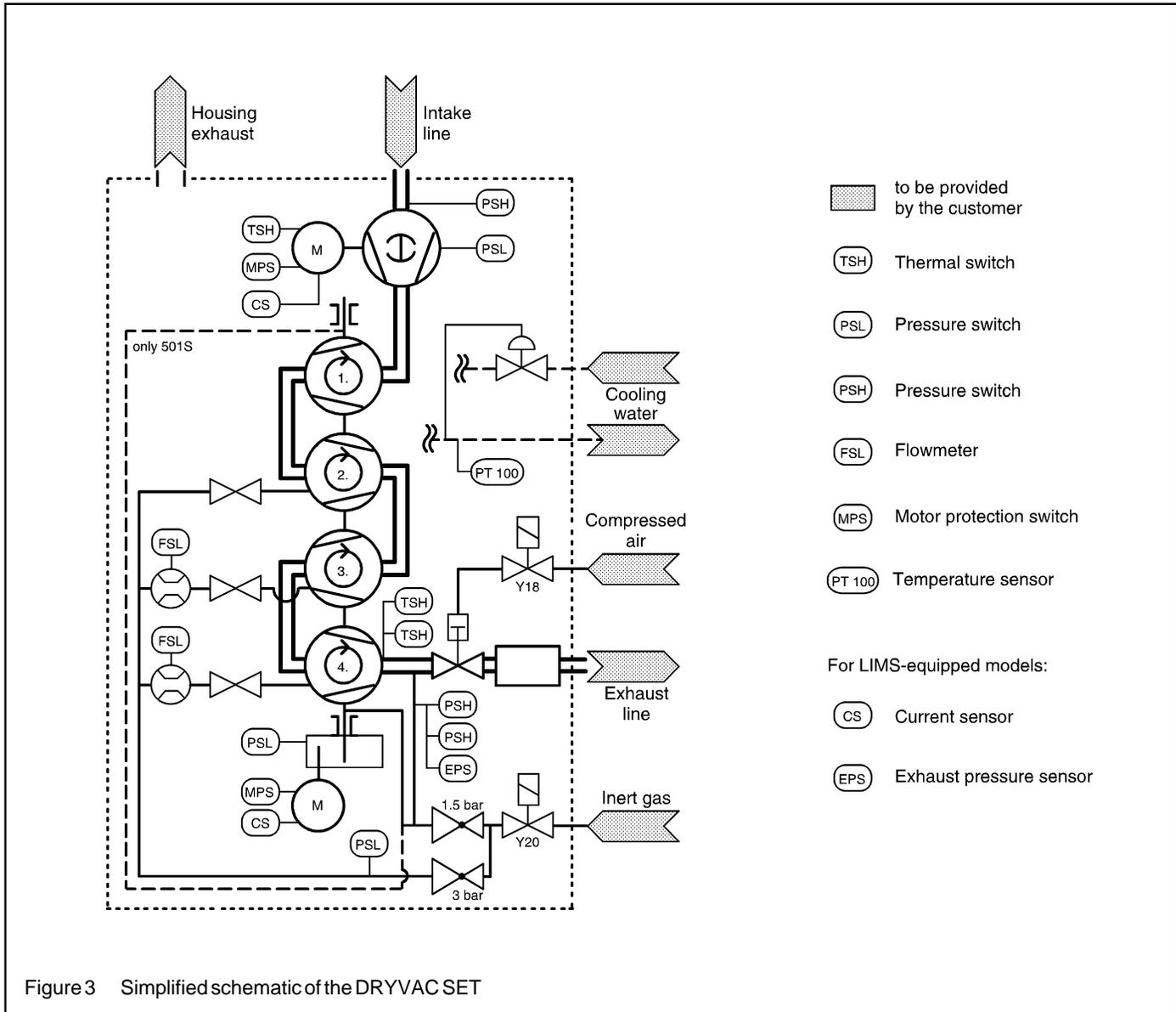
Figure 3 Simplified schematic of the DRYVAC SET
