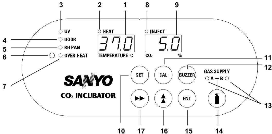
1. **Digital temperature indicator** (TEMPERATURE °C): Normally, this indicator shows the chamber temperature. In the setting mode, it shows the set value of the chamber temperature. If the self diagnostic function detects any abnormality, an error code will be displayed.
