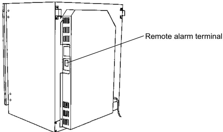
The remote alarm terminal is a contact output.
