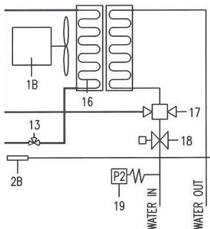
*Cooltechnical pattern of a SCANCOOL freezer incl. water cooled condenser.*
