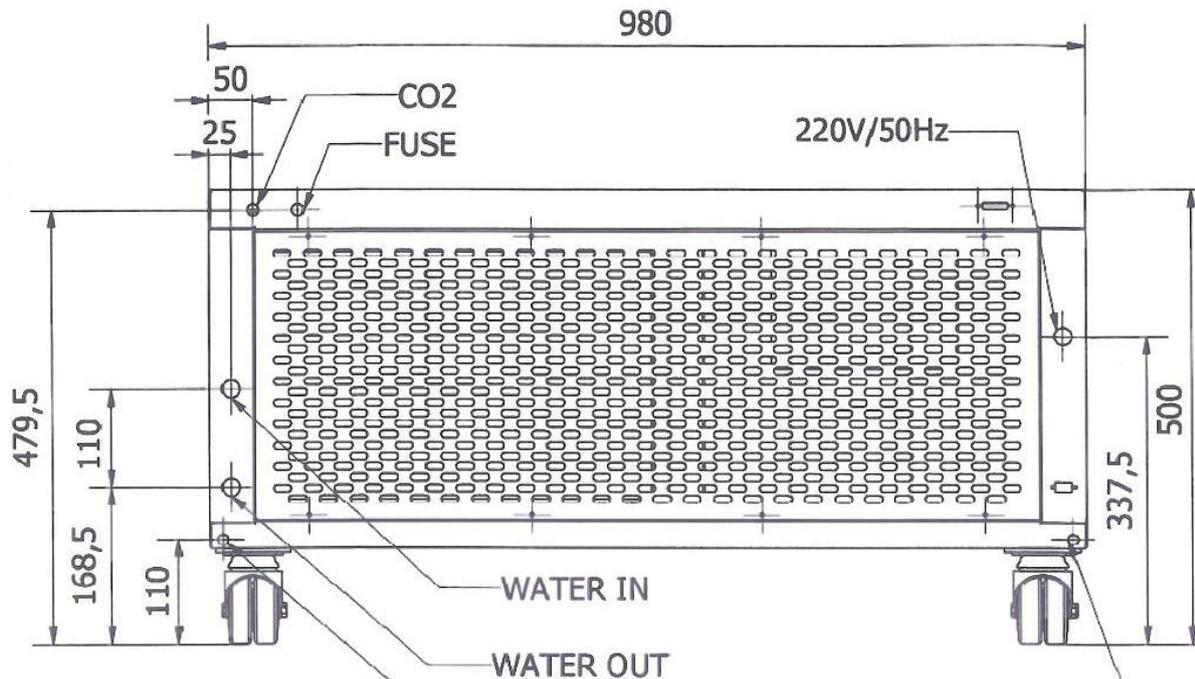
*(4) backside of the freezer, type SCL610P, connections for watercooling, connection to CO<sub>2</sub> back-up cooling system*
