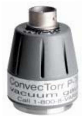
Designed as a vacuum atmosphere simulator for multigauge and sentorr tube to be used with any of the controllers that can accept a 531 thermocouple gauge tube. For those applications where the TC tube will never see  $1 \times 10^{-3}$  torr, it serves as an ideal reference when adjusting the vacuum (zero) calibration potentiometer on the controller. Troubleshooting is facilitated by the selectable Vac or Atm setting.
