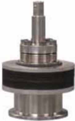
Varian Vacuum Technologies is introducing the Inverted Magnetron Cold Cathode transducer (IMG), a cold cathode gauge with controlled magnetic field in the ion chamber. This transducer is capable of reading from  $10^{-3}$  torr ( $10^{-3}$  mbar) down to  $10^{-11}$  torr ( $10^{-11}$  mbar) range. Its linear response and repeated quick ignition characteristic of typically <50 seconds in the  $10^{-11}$  range are well appreciated features of this transducer.
