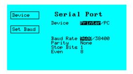
Clicking on the "Device" function key will toggle between Printer and PC.
